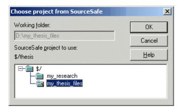
The selected file, its folder, and all files in the folder, are associated with the source control system project you selected. For the example, MATLAB associates all files in D:\my\_thesis\_files with the source control project my thesis files.
