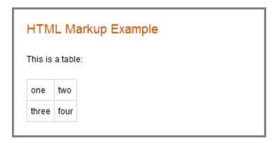
If a section produces command-window output that starts with <html> and ends with </html>, MATLAB includes the source HTML in the published output. For example, MATLAB displays the disp command and makes a table from the HTML code if you publish this code:
